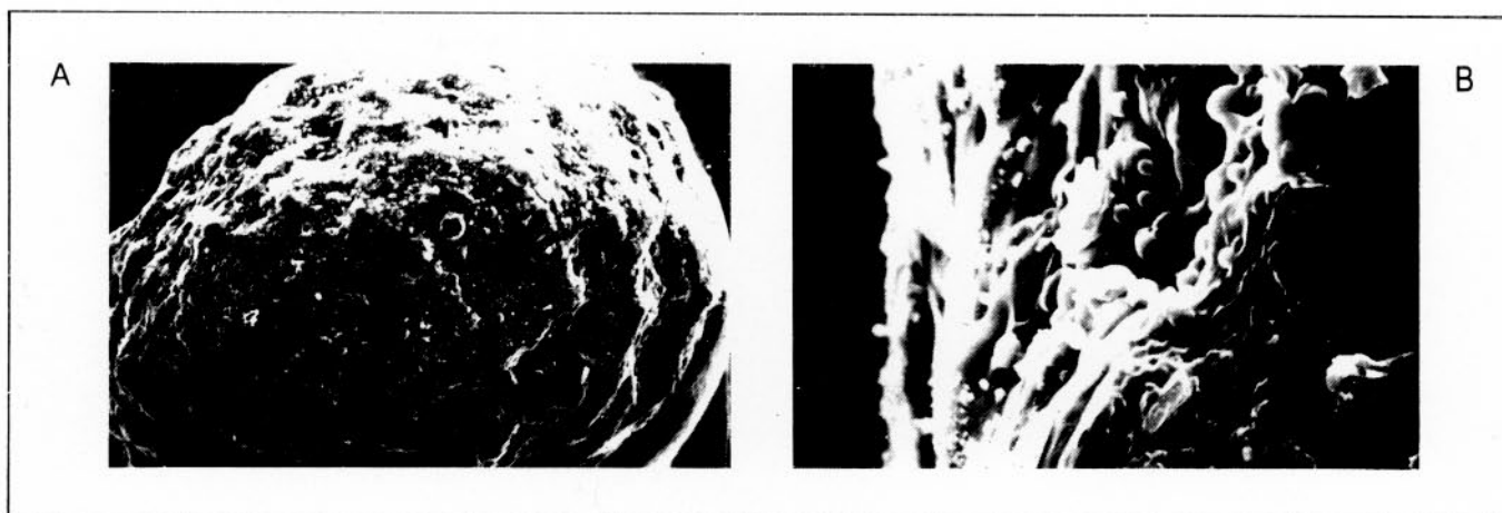
Figure 2: Pellets coated using an aqueous system in a modified perforated pan (A: magnification = 100X; B: cross section, magnification = 1500X).
